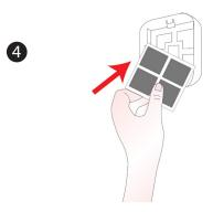
Remove and discard the old filter which is located on the inside of the filter cover.
